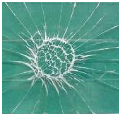
Fig. 3: The Glass After the Test
