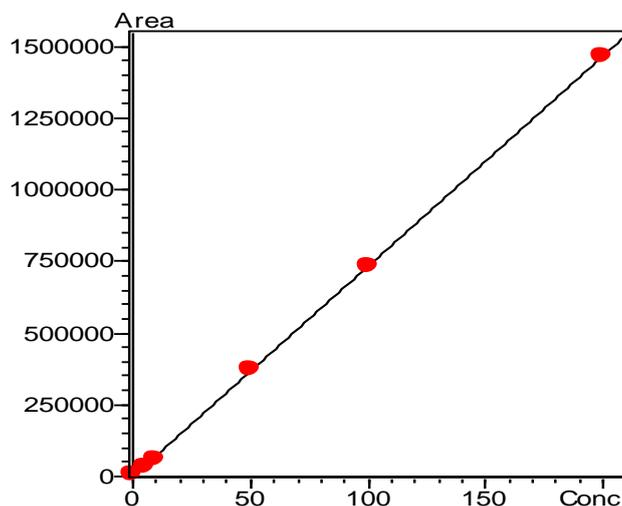
**Figure 2:** Calibration curve of choline ( $\mu\text{g/L}$ ), 0.5  $\mu\text{g/L}$  ~ 200  $\mu\text{g/L}$  (ppb)
