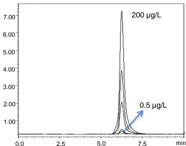
**Figure 1:** LCMS Chromatogram of choline standards in SIM mode ( $m/z$  104.2)
