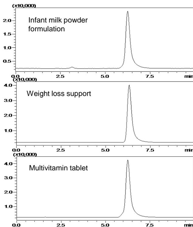
**Figure 3:** Chromatograms of choline in SIM mode (m/z 104.2) in three samples
