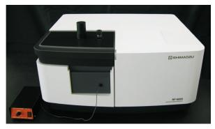
Fig. 1 RF-6000 Spectrofluorophotometer Coumarin (Diesel Oil Marker) Identification System
