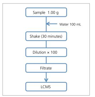
Fig. 3 Preparation Flow
