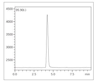
Fig. 1 Mass Chromatogram (SIM) of Sulfamic Acid (0.1 mg/L)
