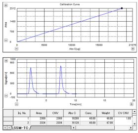
Fig. 4 Measurement Data for Calibration Curve
