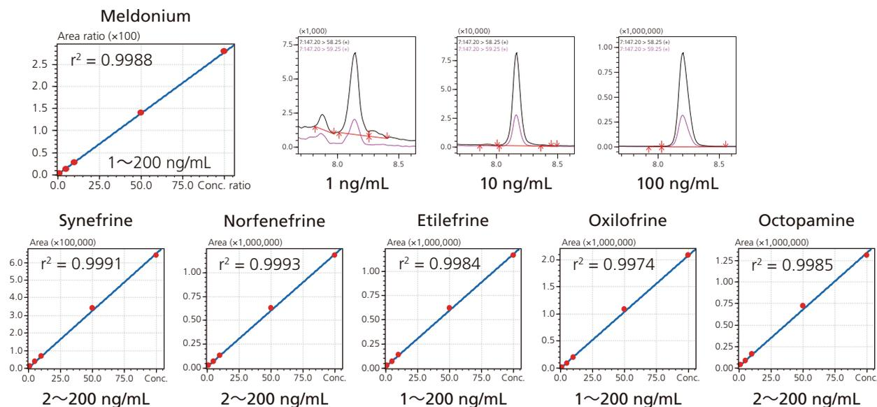
Fig. 4 Calibration Curves and MRM Chromatograms of 6 Compounds
