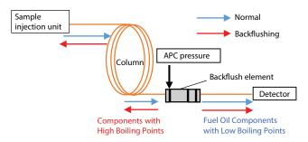
Fig. 1 Overview of Backflush System
