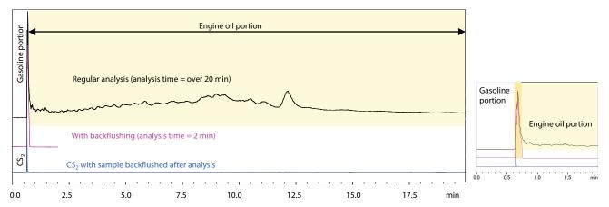
Fig. 3 Chromatogram of Engine Oil Containing Gasoline
