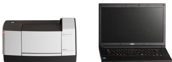
Fig. 1 Appearance of IRSpirit, a Compact FTIR
