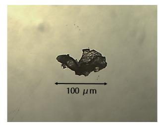
Fig. 2 Stereo Microscope Image of Contaminant
