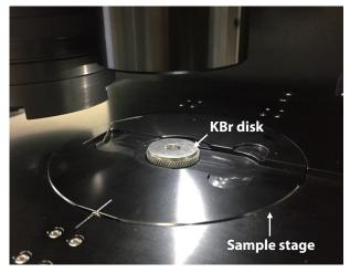
Fig. 4 KBr Disk Set for Measurement
