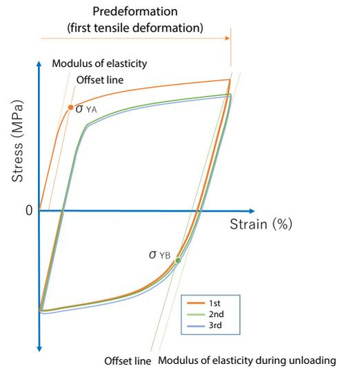
Fig. 2 Conceptual Diagram of Bauschinger Effect Evaluation Results
