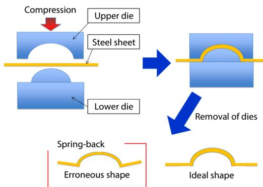
Fig. 1 Spring-back Phenomenon in Steel Sheet Forming
