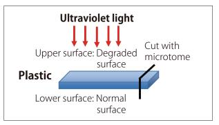
Fig. 1 Flat Cross-Sections from Degraded PP Plastic
