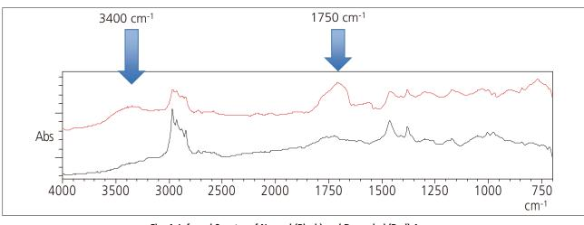
Fig. 4 Infrared Spectra of Normal (Black) and Degraded (Red) Areas
