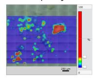
Fig. 6-(c) PET Distribution (Based on the corrected peak height value of 1724 cm<sup>-1</sup>)
