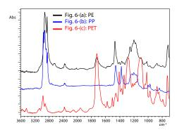
Fig. 7 Typical Infrared Spectra from Areas in Figs. 6-(a) to (c)  $\,$
