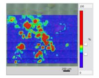
Fig. 6-(a) PE Distribution (Based on the corrected peak height value of 718 cm<sup>-1</sup>)
