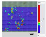
Fig. 6-(b) PP Distribution (Based on the corrected peak height value of 2839 cm<sup>-1</sup>)
