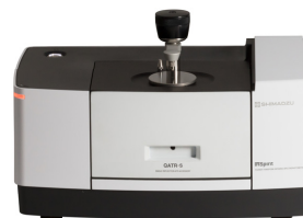
Fig. 3 QATR-S ATR accessory mounted in IRSpirit
