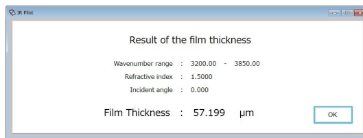
Fig. 7 Result of Film Thickness Determination
