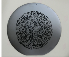
Fig. 3 Test Specimen Showing Random Pattern
