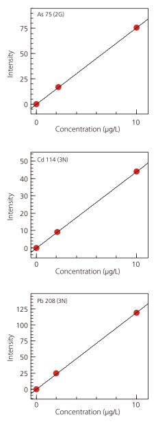
Fig. 1 Calibration Curves for As, Cd and Pb
