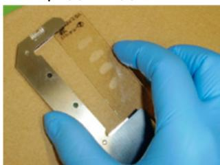
Fig. 8 Inserting the Microscope Slide into the Sample Holder
