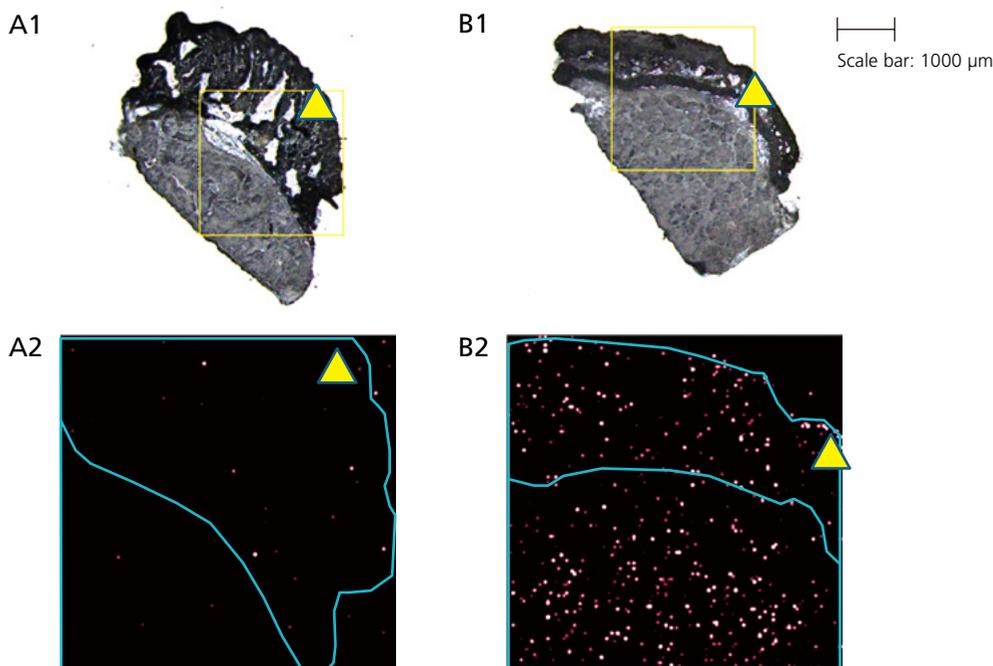
Fig. 7 MS/MS Imaging (Upper: Optical Images, Enclosed Areas Were Analyzed; Lower: MS/MS Images from  $m/z$  892.3 to 607.19)
