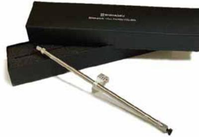
LC Column : Shim-pack GIS C18 (3.0 mm x 150 mm, 3 μm)
