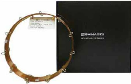
GC Column : SH-I-5Sil MS (0.25 mm x 30 m , 0.25 μm)
