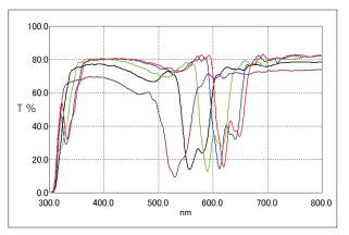
Fig. 10 MLF-19 Film Transmission Spectra
