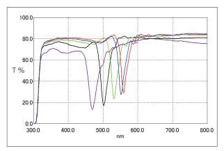
Fig. 8 MLF-16.5 Film Transmission Spectra
