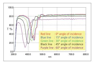
Fig. 5 MLF-13.0 Film Transmission Spectra
