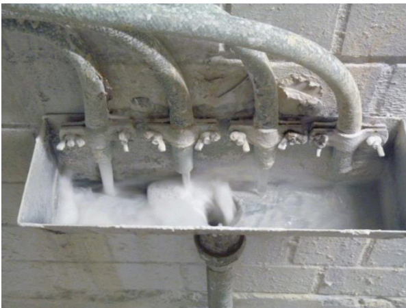
Fig.: Example from paper industry: Four very diverse sample streams
