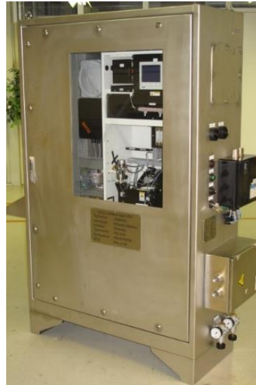
Fig.: TOC analyser in pressurized cabinet
