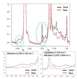
Fig.4(a) Infrared Spectra of New and Used Lubricant A
