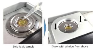
Fig. 3 Sample Setting Procedure
