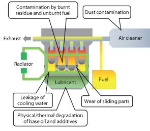
Fig. 1 Representative Causes of Lubricant Degradation in Engines
