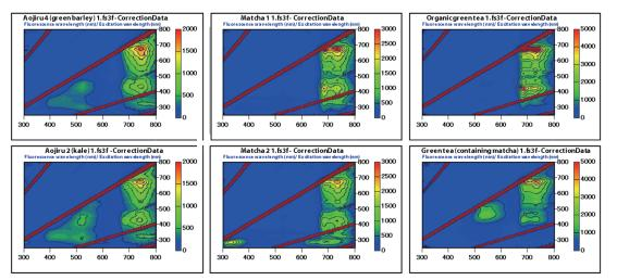
Fig. 5 3D Fluorescence Spectra of Powder Samples
